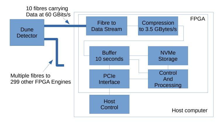
lock a particular chunk in NVMe storage against subsequent writes if it contains data of interest. The data from this chunk can then be read out by the host computer.
