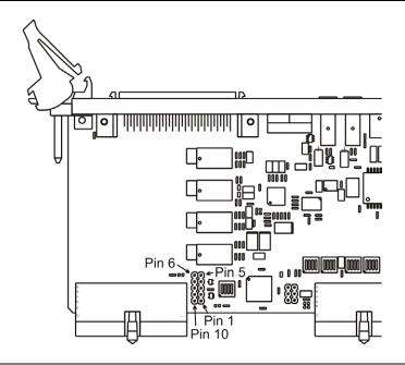
Figure A-6 Serial Interface (LK4) Header
