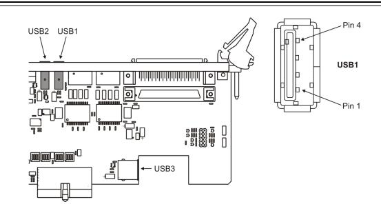
Figure A-4 USB1 (P2) and USB2 (P1) Connectors
