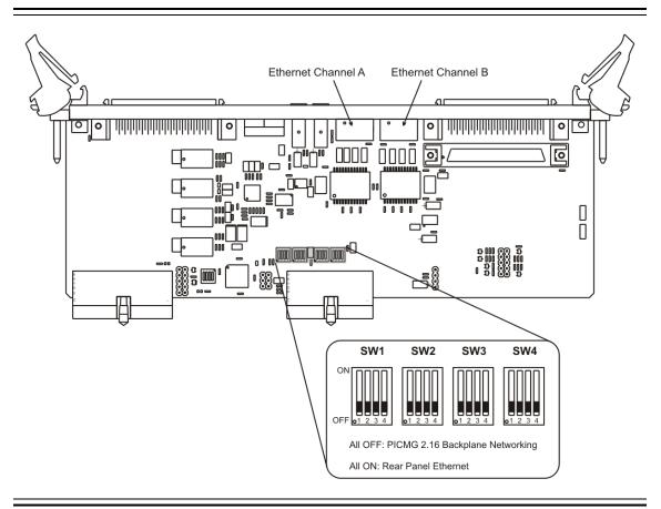
Figure 2-3 Ethernet DIL Switches
