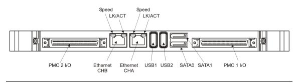
Figure A-3 Front Panel Connector Layout
