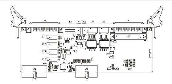
Figure A-2 Connector Layout (Rev A boards)
