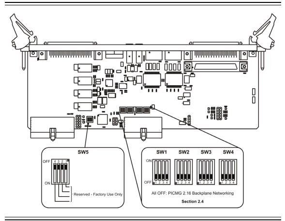
Figure 2-2 Factory Switch Settings (Rev A boards)
