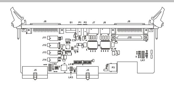
Figure A-1 Connector Layout (Rev B and Rev C boards)
