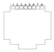
Figure A-5 Ethernet RJ45 Connector (Front View)
