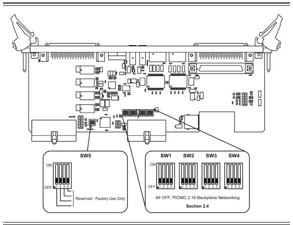
Figure 2-1 Factory Switch Settings (Rev B and Rev C boards)
