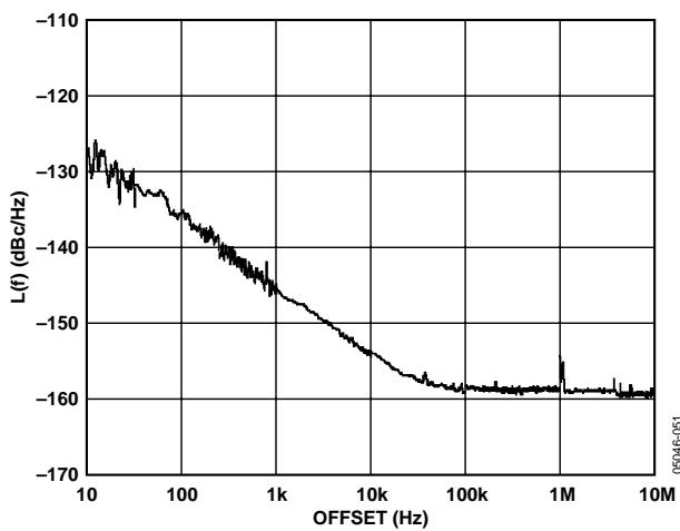
Figure 24. Additive Phase Noise—LVPECL DIV 1, 245.76 MHz;
