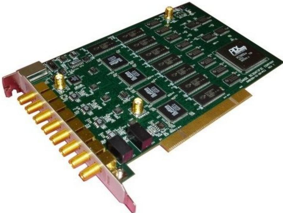
Each of the boards 8 outputs provides 2Volts peak to peak into 50 Ohm's through an SMA connector. There is also a TTL Marker output. This has been used to drive the CYCLE\_STOP signal. The channels are allocated as follows:
