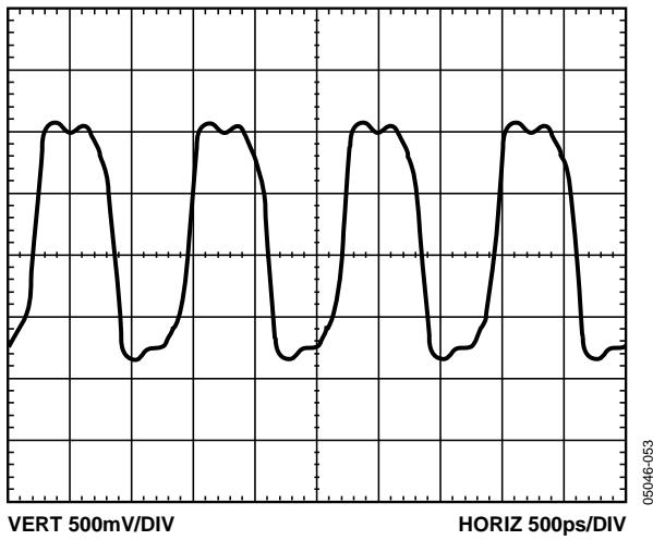
Figure 18. LVPECL Differential Output @ 800 MHz
