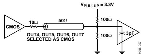
Figure 55. CMOS Output with Far-End Termination
