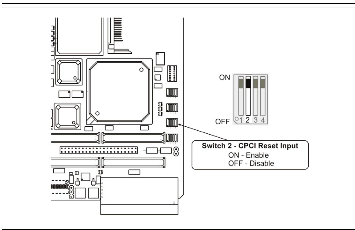
Figure 2-15      CompactPCI Reset Input Switch
