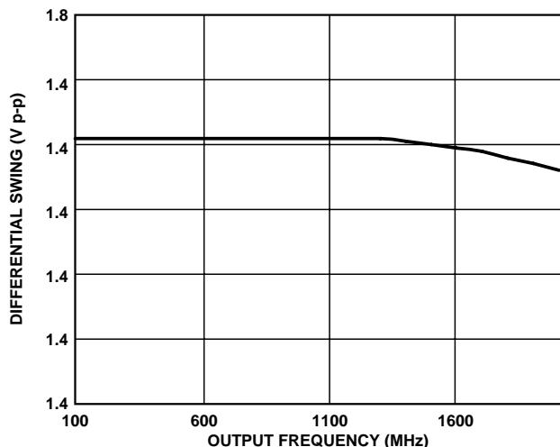
Figure 21. LVPECL Differential Output Swing vs. Frequency
