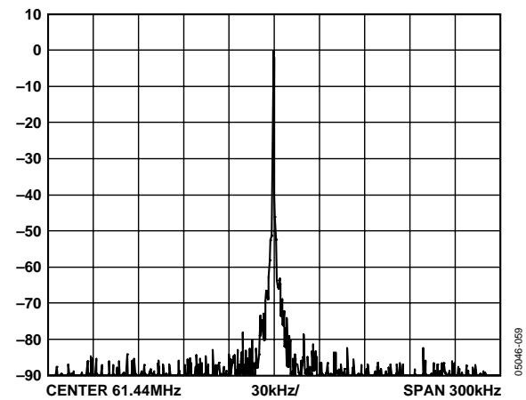
Figure 15. Phase Noise, LVPECL, DIV 4, FVCXO = 245.76 MHz,
