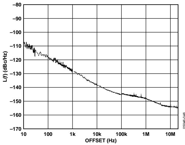
Figure 25. Additive Phase Noise—LVDS DIV 1, 245.76 MHz
