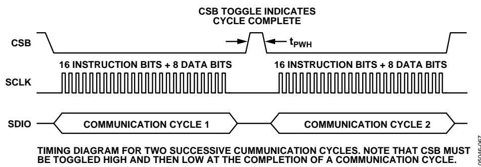
Figure 52. Use of CSB to Define Communications Cycle
