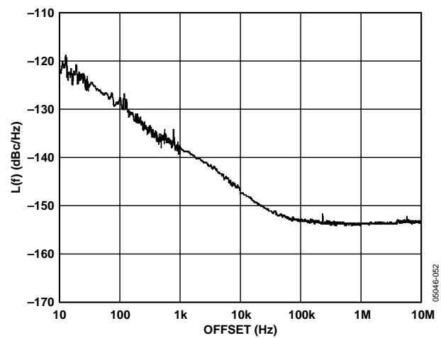
Figure 27. Additive Phase Noise—LVPECL DIV1, 622.08 MHz
