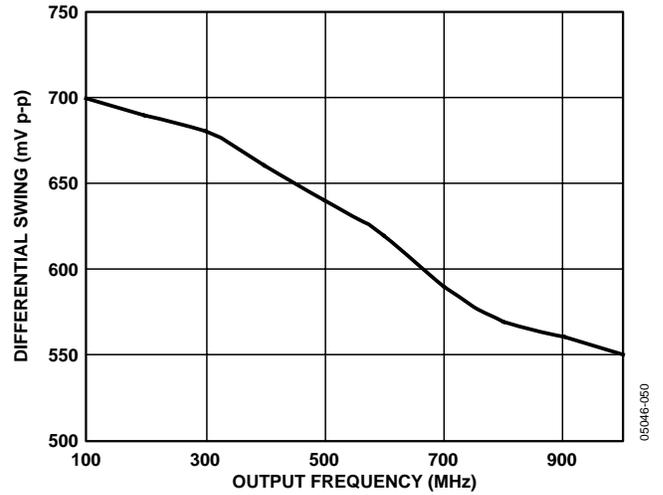
Figure 22. LVDS Differential Output Swing vs. Frequency
