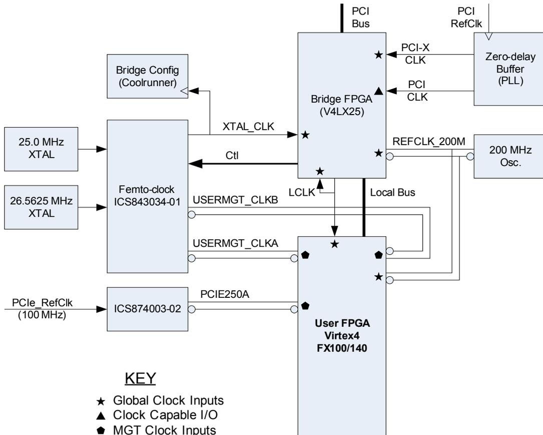
Figure 3 FPGA Logic Clock Distribution
