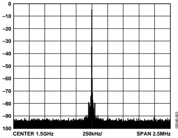
Figure 13. PLL Reference Spurs: VCO 1.5 GHz, FPF = 1 MHz
