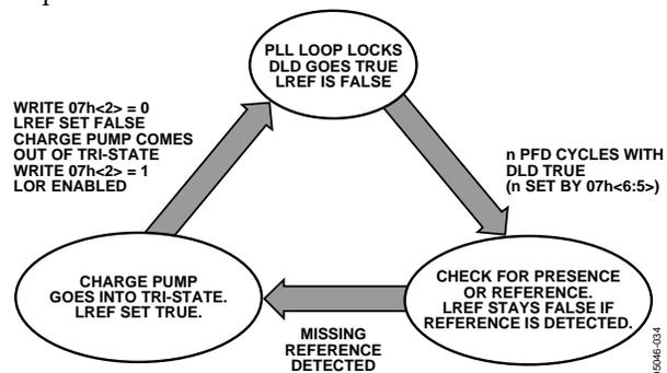
Figure 38. Loss of Reference Sequence of Events
