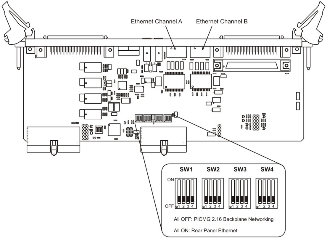
**Figure 2-3 Ethernet DIL Switches**
