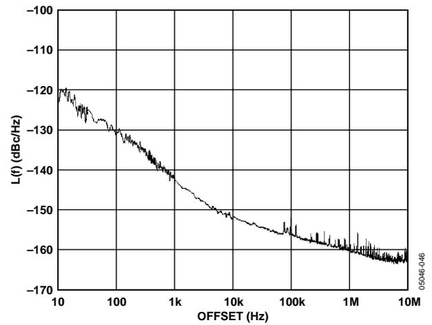
Figure 29. Additive Phase Noise—CMOS DIV4, 61.44 MHz
