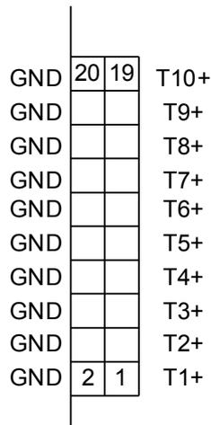
Figure 5 Front Panel Timing Bus
