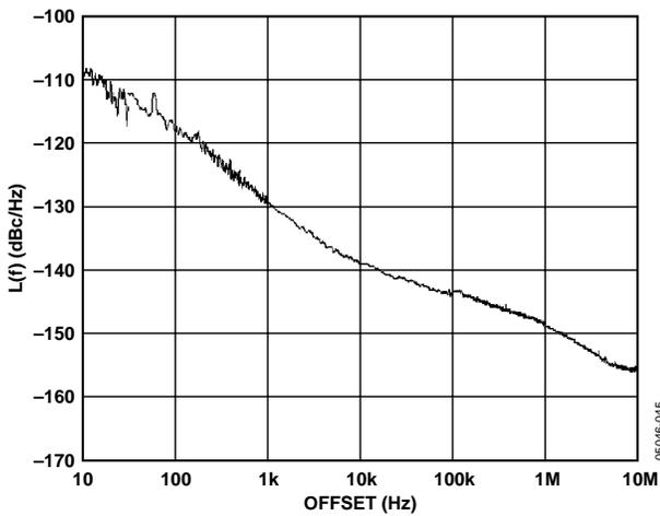
Figure 26. Additive Phase Noise—CMOS DIV 1, 245.76 MHz
