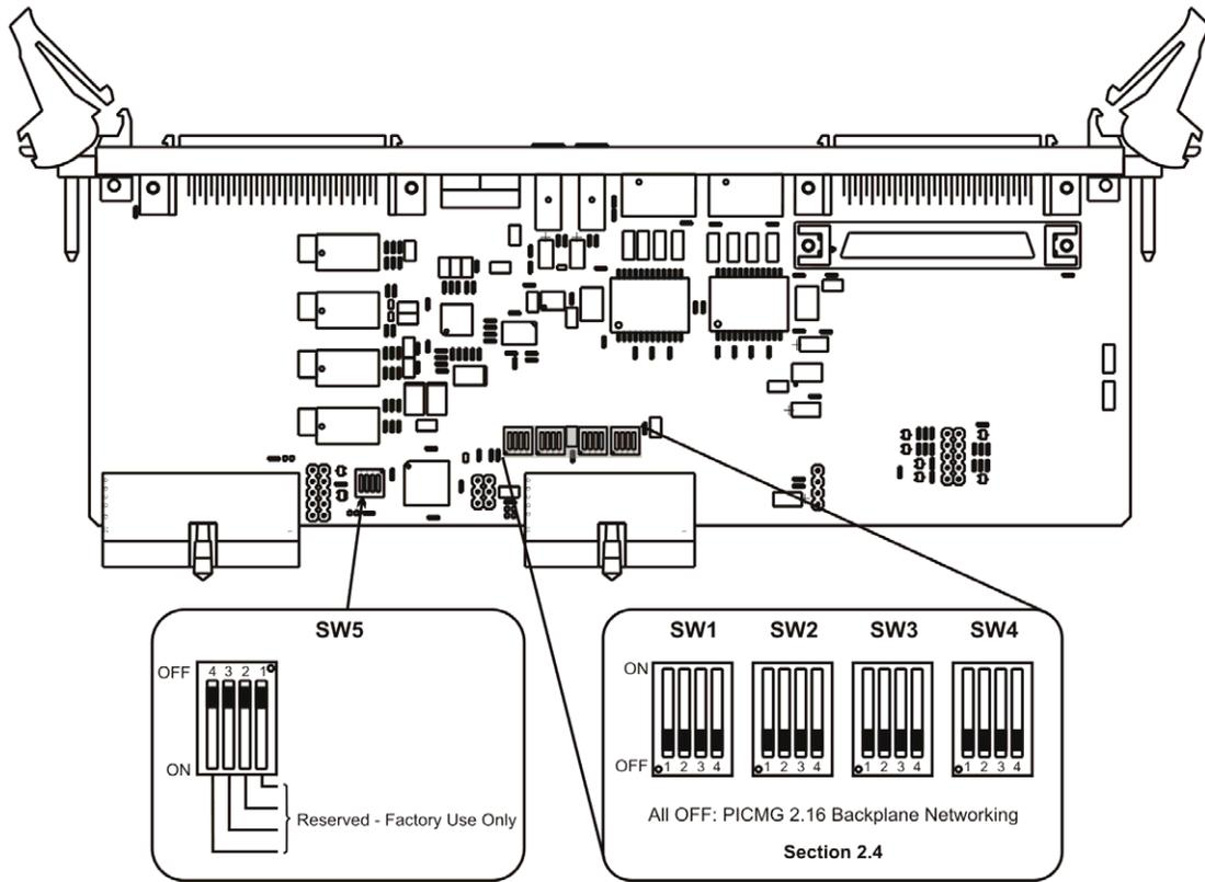
**Figure 2-2** Factory Switch Settings (Rev A boards)
