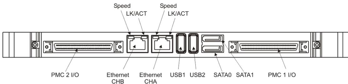
**Figure A-3 Front Panel Connector Layout**
