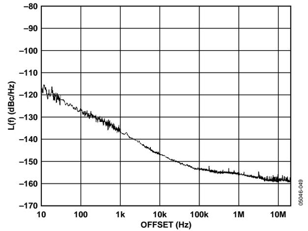
Figure 28. Additive Phase Noise—LVDS DIV2, 122.88 MHz
