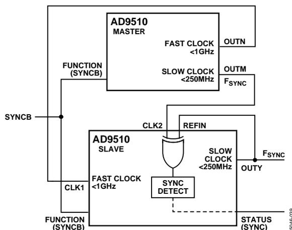
Figure 43. Multichip Synchronization
