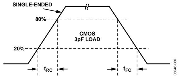
Figure 5. CMOS Timing, Single-Ended, 3 pF Load
