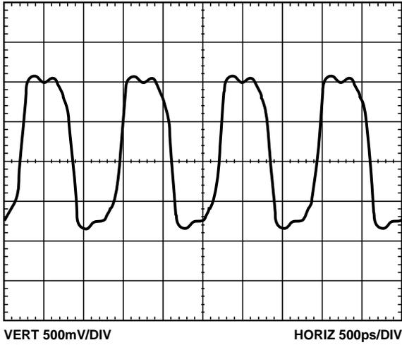
Figure 18. LVPECL Differential Output @ 800 MHz
