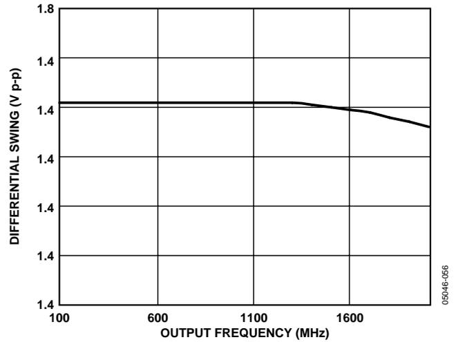
Figure 21. LVPECL Differential Output Swing vs. Frequency
