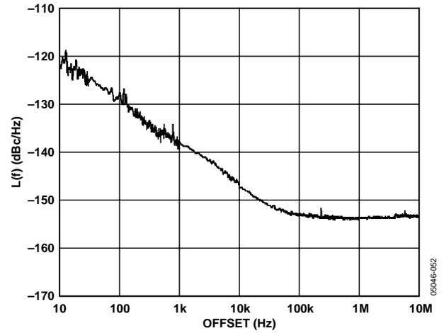
Figure 27. Additive Phase Noise—LVPECL DIV1, 622.08 MHz
