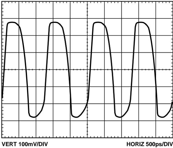
Figure 19. LVDS Differential Output @ 800 MHz
