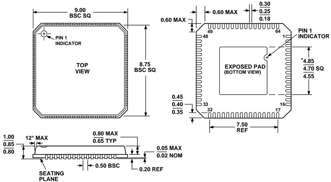
\*COMPLIANT TO JEDEC STANDARDS MO-220-VMM D EXCEPT FOR EXPOSED PAD DIMENSION
