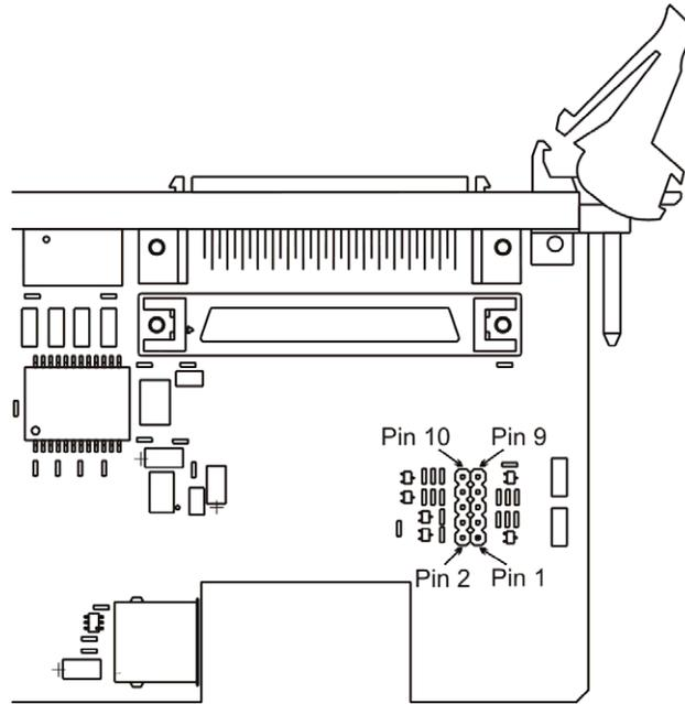
**Figure A-7** General Purpose I/O (LK1) Header (Rev B and Rev C boards)
