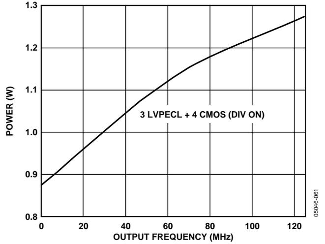
Figure 10. Power vs. Frequency—LVPECL, CMOS (PLL Off)
