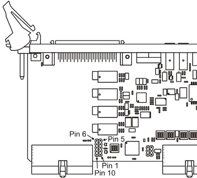
**Figure A-6 Serial Interface (LK4) Header**
