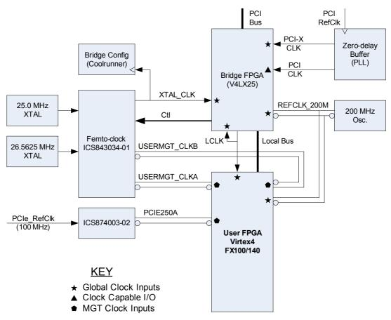
Figure 3 FPGA Logic Clock Distribution
