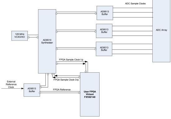
Figure 4 Sampling Clock Distribution
