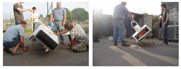
The angle at the balance point was 43 degrees. We also measured the weight on the front and rear tyres and tested the sideways tyre friction on tarmac. These were:
