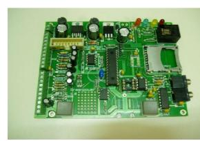
We designed a simple PIC micro based Car Computer board that could be easily built by the pupils and would perform all of the data gathering and logging functions we desired. The PCB was tracked by a parent with some pupil input using the kicad free PCB package. In order to improve reliability, (and make it easier for ourselves to build !), we had 6 PCB's manufactured professionally on double sided boards.
