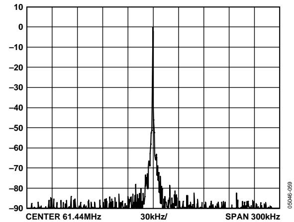
Figure 15. Phase Noise, LVPECL, DIV 4, FVCXO = 245.76 MHz,
