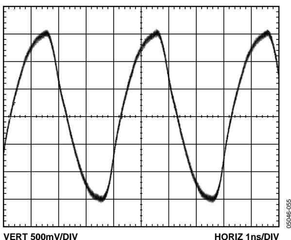
Figure 20. CMOS Single-Ended Output @ 250 MHz with 10 pF Load
