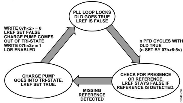
Figure 38. Loss of Reference Sequence of Events
