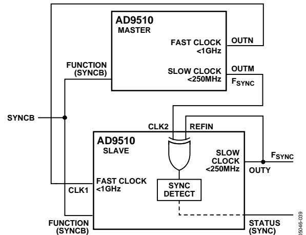
Figure 43. Multichip Synchronization
