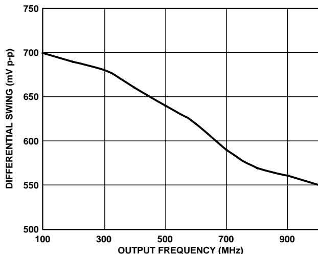
Figure 22. LVDS Differential Output Swing vs. Frequency
