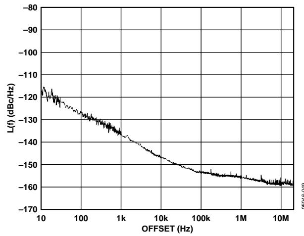
Figure 28. Additive Phase Noise—LVDS DIV2, 122.88 MHz
