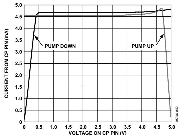
Figure 17. Charge Pump Output Characteristics @ VCPs = 5.0 V
