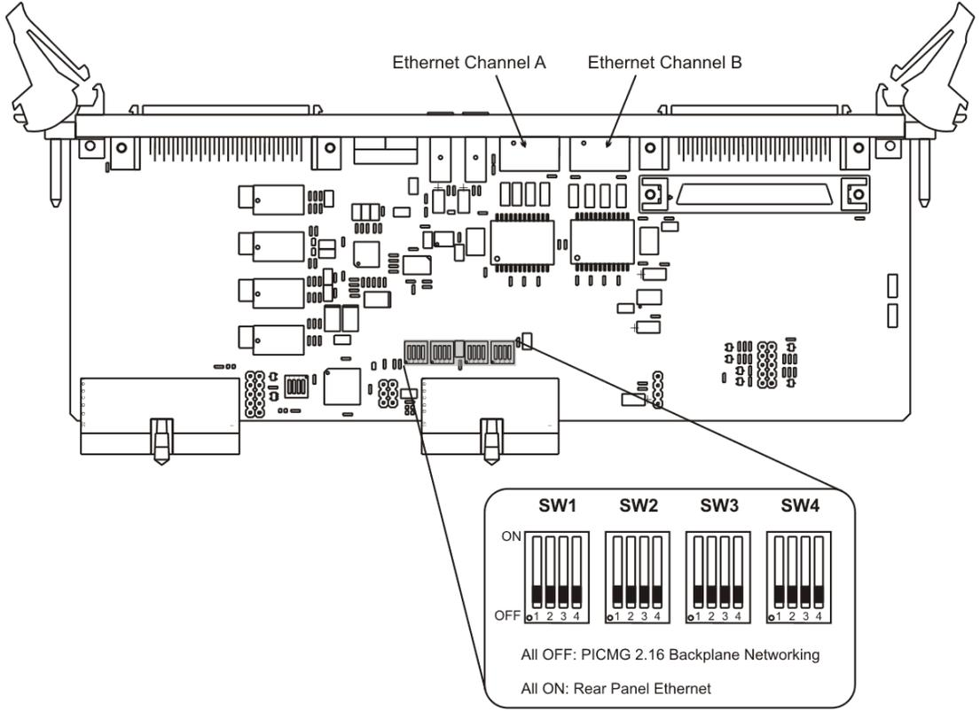
**Figure 2-3 Ethernet DIL Switches**
