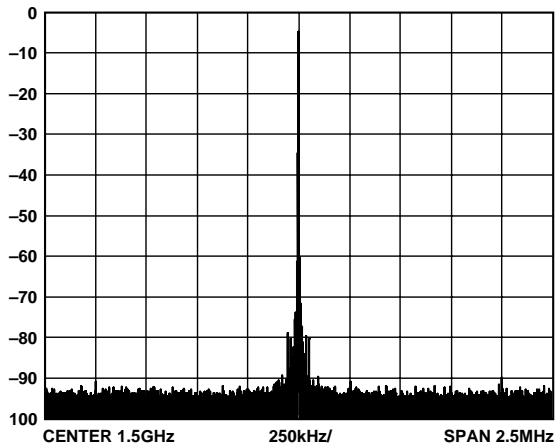
Figure 13. PLL Reference Spurs: VCO 1.5 GHz, FPFD = 1 MHz
