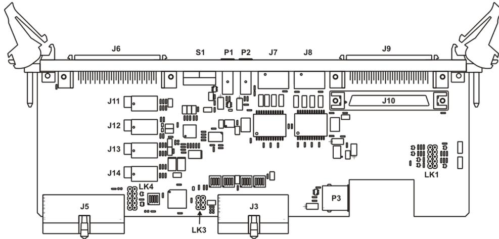
**Figure A-1 Connector Layout (Rev B and Rev C boards)**
