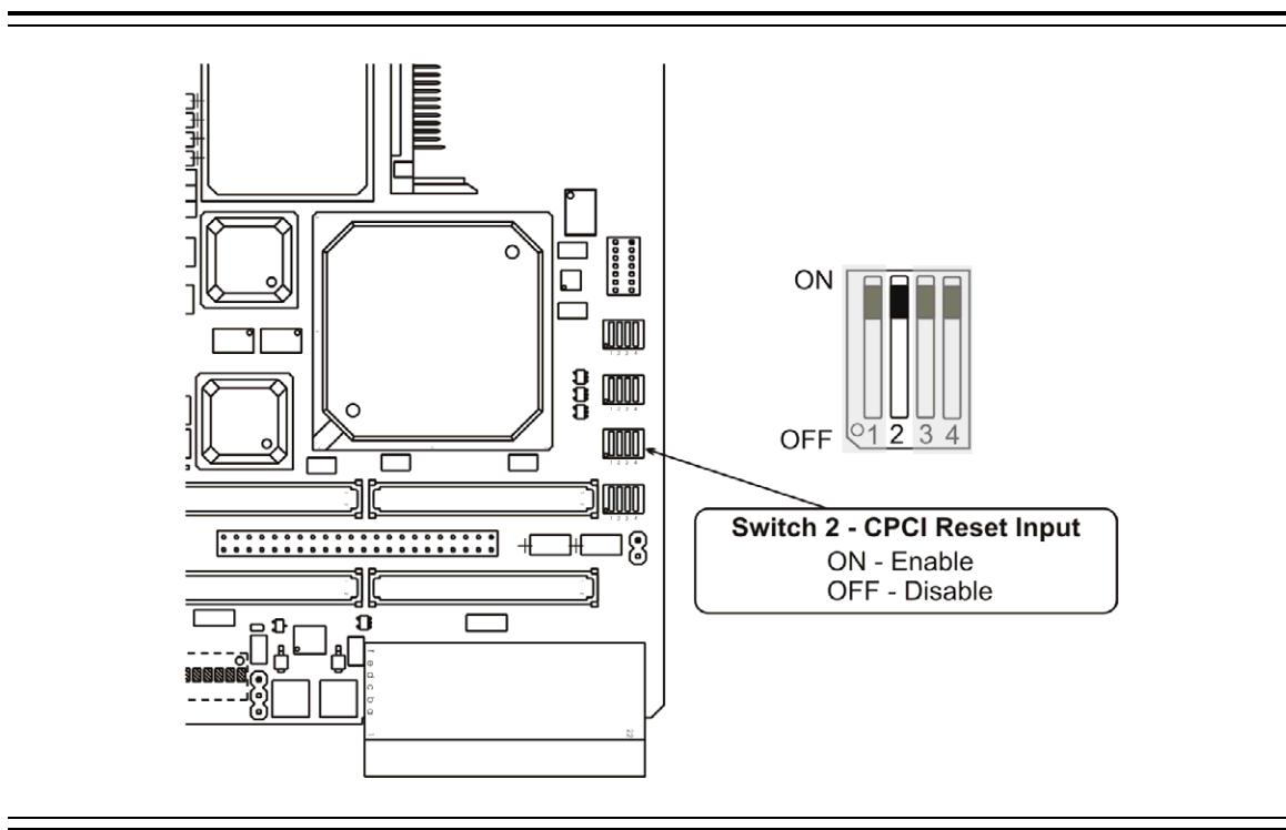
Figure 2-15      CompactPCI Reset Input Switch
