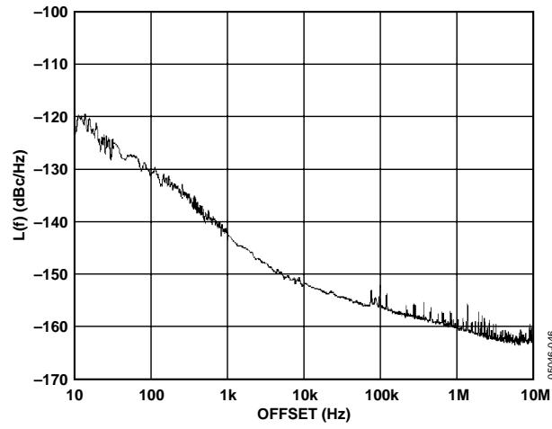
Figure 29. Additive Phase Noise—CMOS DIV4, 61.44 MHz
