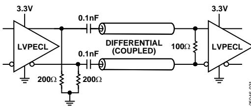
Figure 57. LVPECL with Parallel Transmission Line
