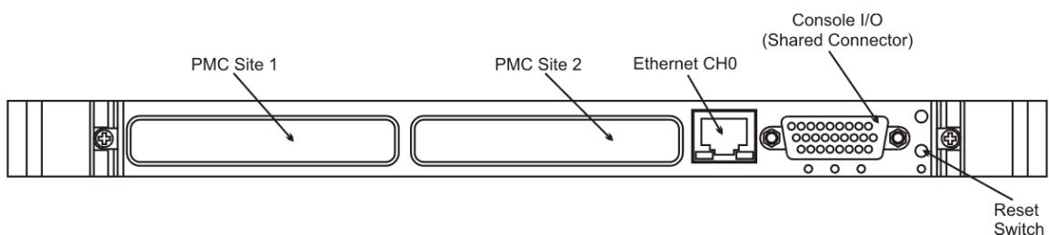
Figure A-2      Front Panel Connectors
