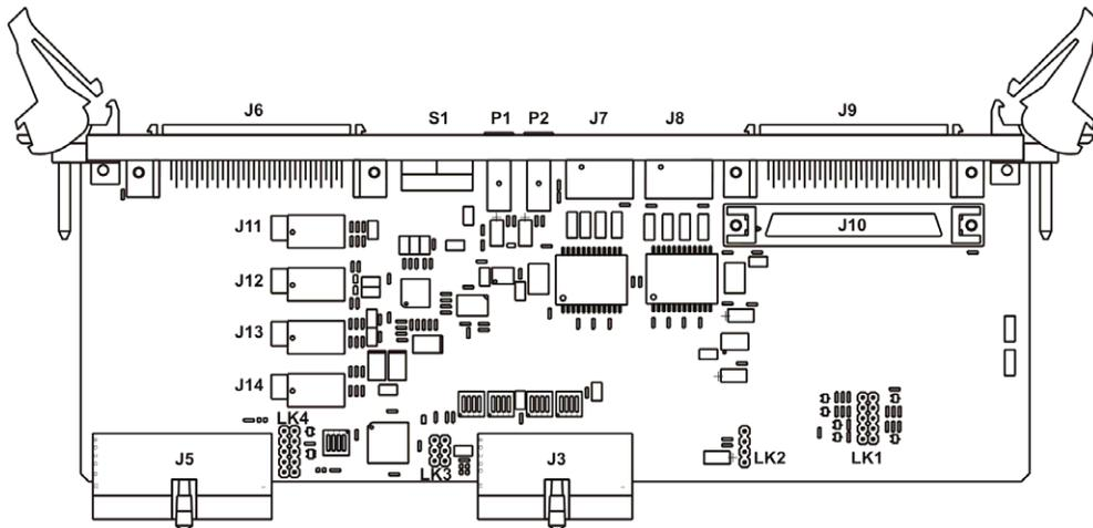
**Figure A-2 Connector Layout (Rev A boards)**
