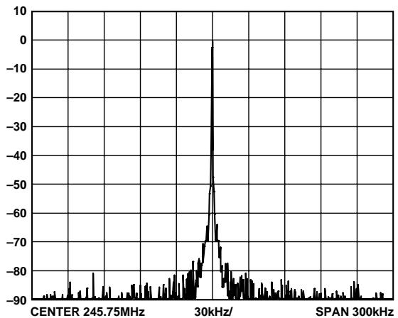
Figure 12. Phase Noise, LVPECL, DIV 1, FVCXO = 245.76 MHz,
