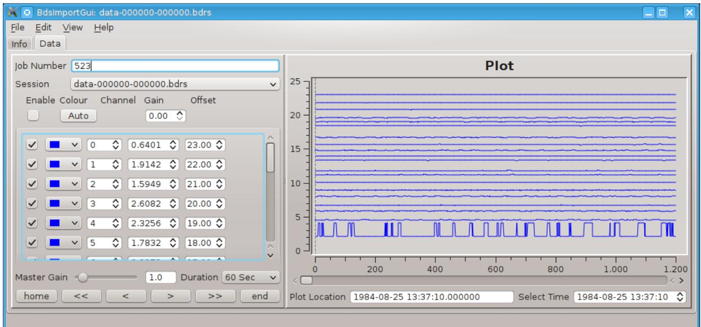
The data tab displays the waveform data channels of the bdrs session file. Controls are provided to navigate the data. The "Plot Location" time shown below the waveforms is the sample time of the leftmost sample currently displayed.
