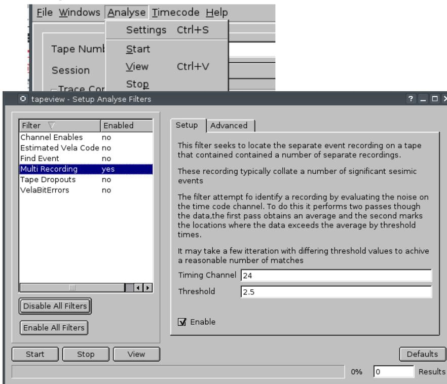
The available filters are displayed in a list. Analysis may started and stopped and the results of viewed within the results viewer. To enable a filter either double click on the filter in the filter list or check the enable checkbox. Start the analysis by clicking on the start button. When complete click the view button to view the results. The Setup tab displays the options available to each filter.
